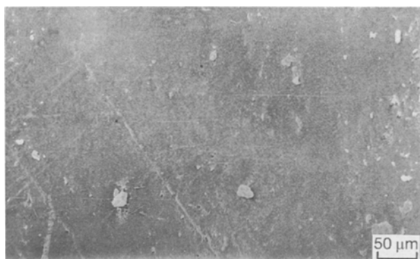
Figure 2 SEM photograph of 50:50 conventional blend (mix A).
