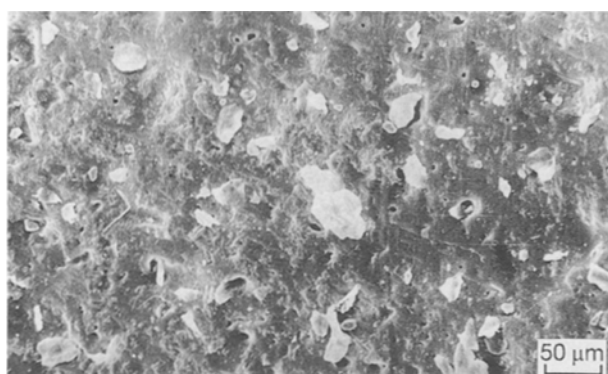
Figure 1 SEM photograph of 50:50 particulate blend (mix D).
